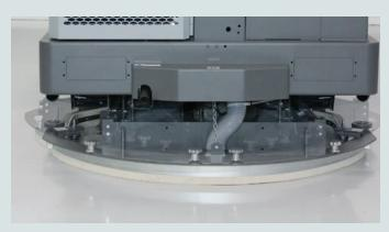
Patented Accu-Track<sup>™</sup> squeegee provides superior water pick-up even during the tightest turns.
