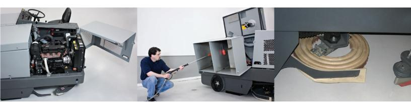
Maintenance is a breeze with easy-toreach engine, electrical and hydraulic components.
