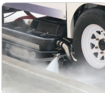
Integrated curb cleaner for the vertical faces of curbs.
