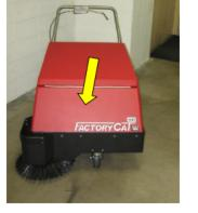
The 34 sweeper is a 12 volt machine with high quality "Trojan" brand industrial batteries and therefore can offer longer run time than machines with smaller amp hour batteries. Properly equipped, the 34 can operate for almost a full shift and clean over 34,000 square feet on a charge.
