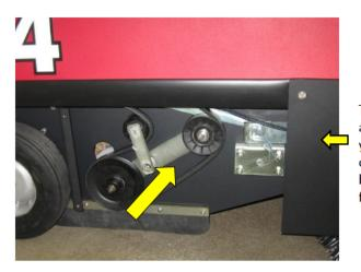
The 34 sweeper uses a single powerful motor to run the fan and broom. This 1 hp motor directly generates maximum cfm for dust control and is sealed for long life. It powers the main broom through a HD belt, allowing slippage in the event the broom is run over potentially damaging obstacles.
