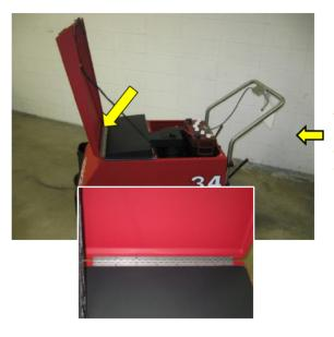
The 34 sweeper uses a large stainless hinge for the hood that bolt directly to the steel frame. This provides better durability than other machines that use smaller hinges bolted to plastic frames.
