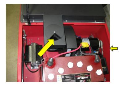
A feature to 34 sweeper is the Wet Sweep ByPass door. The operator can simply rotate this cover open to reduce the airflow into the filter when water on the ground is encountered.
