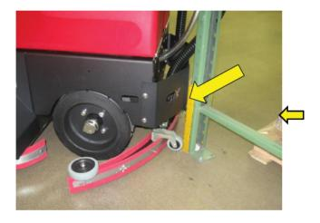
Our GTX scrubber comes standard with a heavy-duty steel rear bumper, which helps protect the squeegees in "reverse" collisions. All scrubbers offer "breakaway" squeegees for "forward" collisions.
