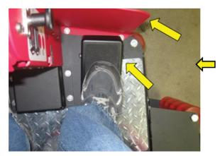
The GTX scrubber has a simple and large pedal, which controls speed. This view also shows the protection offered to the Operator's foot on the GTX scrubber. A complete apron across the front makes it harder for the operator to hang his foot off the side, reducing potential injuries.
