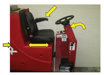
The heavy duty wide steel frame of the GTX scrubber offers stability without the need for tip-over bars used on some other machines.
