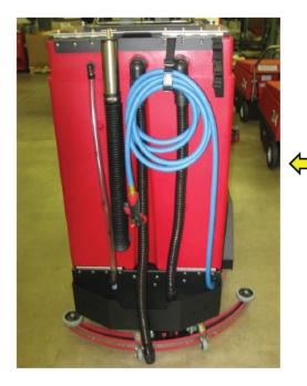
Spray Jet option equips the scrubber with a heavy duty hose 4' - 10' and spray nozzle. This allows the operator to use the scrubber's clean solution under pressure (3.0 gpm / 45 psi) to flush out the recovery tank when draining the tank when fresh water source is not within reach. Operator can also cleanout the scrub deck/hopper, pre-spray a large floor area for better detergent dwell time, cleaning under racks, around equipment, into restrooms and more.
