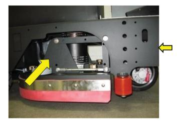
The GTX scrubber mounts its solution valves in the Top Side Service, axle mount. This keeps the solution valves cleaner and free of debris than solution valves mounted on the scrub deck.
