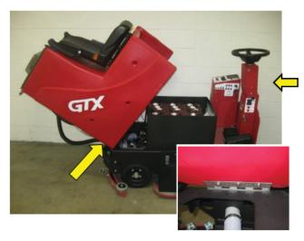
The GTX scrubber uses larger (8" stainless) hinges and bolt directly into the heavy gage steel frame. This provides better durability than other machines that use smaller tank hinges bolted to plastic tanks.
