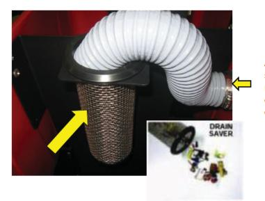
A feature to GTX scrubber is the "Drain Saver" stainless steel basket that collects litter from recovery water. This reduces the potential of discharge water clogging the customers' floor drains. A simple device that can avoid costly drain repairs for customers.
