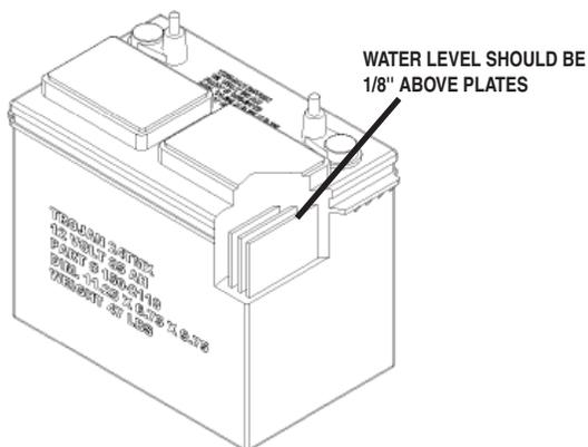
2. Clean Battery tops to prevent corrosion.
