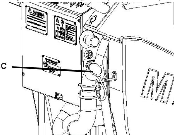
3. Flush Recovery Tank with water hose.
