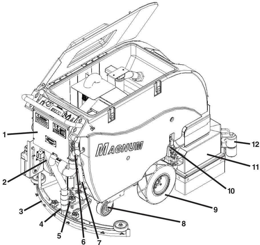
1. **CONTROL PANEL:** Machine controls and access to electrical components
