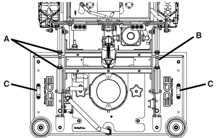
6. Extending the Adjustable Arms raise the front and lowers the rear of the Scrubdeck. After Scrubdeck has been leveled - tighten Locking Nuts (A).
