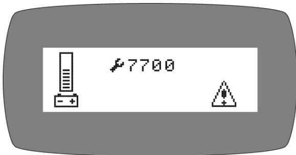
**3. 770, 7701, 7702, and 7703 ERROR:** The vacuum motor has exceeded their authorized power limits. Turn *OFF* Key and turn *ON* again to clear.
