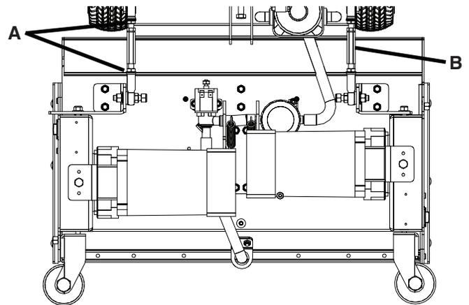
6. Extending the Adjustable Arms raise the front and lowers the rear of the Scrubdeck. After Scrubdeck has been leveled - retighten Locking Nuts **(A)**.
