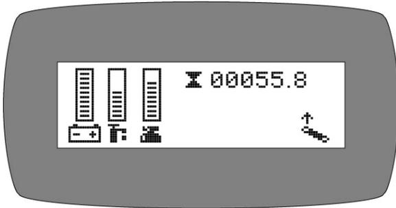
6. **Throttle ERROR:** You pressed the foot pedal before turning on the key. Turn *OFF* the key and try again, leaving foot off of the pedal.
