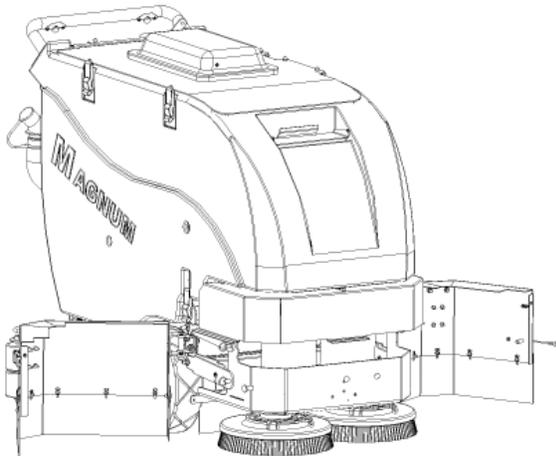
5. Tip Tank Back carefully until supported by strap **(SEE BELOW)**.
