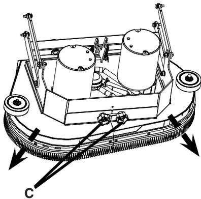
5. Attach Brushes or Pads to Motor Drives. Squeeze the scissor locking device and lift brush up on to the motor drive hub. Make sure the scissors close and lock on the brushes (**SEE BELOW**).
