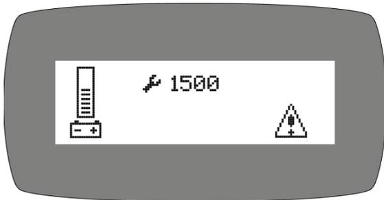
**2. 1500 ERROR:** There is an open in the parking brake circuit. Check the parking brake wiring and the parking brake coil to find the open circuit.
