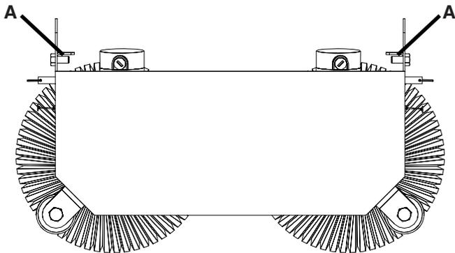
4. To move Side Broom system out of the way when not in use, just pull the pin (**B**) on each side of the Scrubdeck and rotate Side Broom System to the up position and reinsert pin (**SEE BELOW**).
