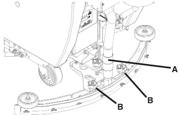
3. Pull Squeegee assembly backward from the lifting carrier.
