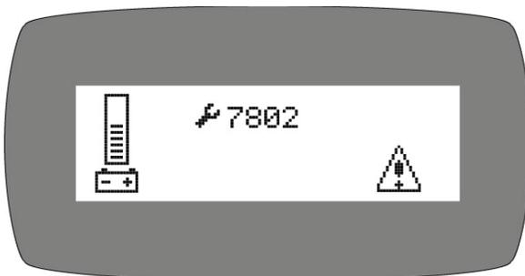
8. **7802 ERROR:** The traction motor pulled excessive current perhaps running a ramp for more than the 60 seconds allowing for this. Turn *OFF* the Key, turn on again, and continue. You should not use this machine to climb ramps so steep and so long that this code comes up repeatedly, or you could overheat the traction motor.
