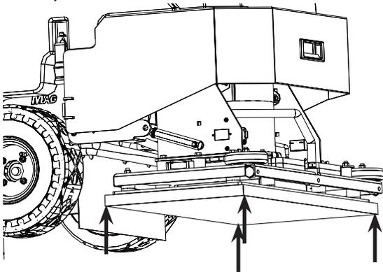
7. With Pad attached securely to Grip Face of EDGE/ORBITZ Deck, the machine is ready to use.
