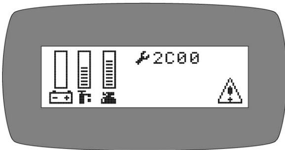
7. **2C00 and 2C01 ERROR:** Low voltage warning. Voltage has dropped down below the minimum required to operate the machine. If you wait a few minutes, the Batteries may come up in voltage, allowing you to drive very slowly to the recharge station. If not, you will have to release the parking brake (on the front wheel, pull lever toward the front of the machine to release) and push the machine to recharging station. You must disconnect the traction motor! (+ cable first)
