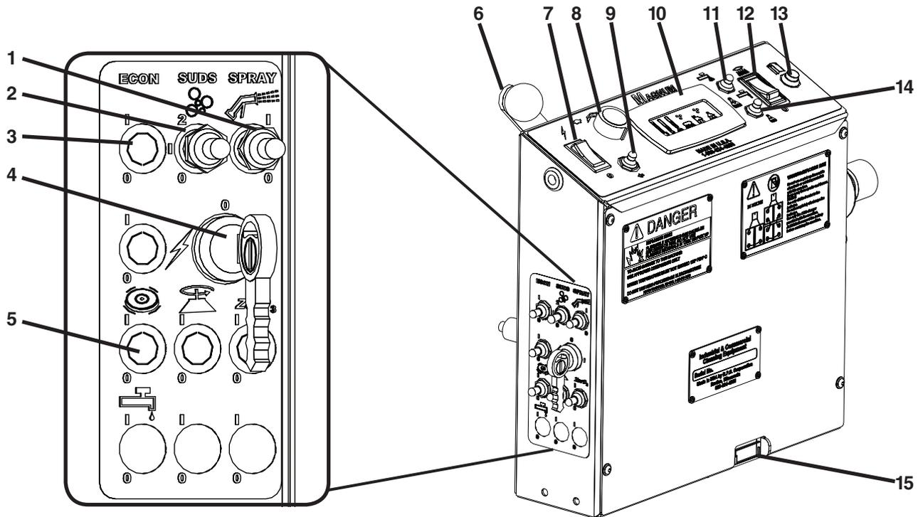
1. **SPRAY JET [BLUE] (OPTIONAL):** Activates Water Pump for remote Spray Wand
