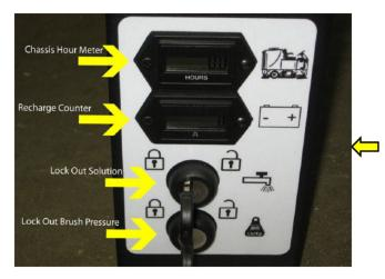
Managers' Lock-Out Brush Pressure allows a Manager, with a private key, to lock out the battery floor scrubber's Scrub pressure adjustment. Our scrubbers offer 5 down pressure settings, and should only be used on maximum settings for floors with heavy soil build up or stripping floor finish. To avoid unnecessary wear on brushes or brushes, this lockout can be employed to maintain Managements' preferred settings.
