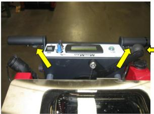
Separate controls for speed and direction, is easy for new operators and in our opinion safer. This system eliminates the possibility that "steering inputs" will affect transport
