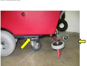
The MiniMag scrubber has a visible and heavy duty steel frame, for durability and protection. All components (casters, transaxle, scrub deck, squeegee linkage and HD jaws all bolt directly to the steel frame.
