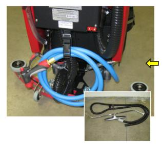
Spray Jet option equips the scrubber with a heavy duty hose 4' - 10' and spray nozzle. This allows the operator to use the scrubber's clean solution under pressure (3.0 gpm / 45 psi) to flush out the recovery tank when draining the tank when fresh water source is not within reach. Operator can also cleanout the scrub deck/hopper, pre-spray a large floor area for better detergent dwell time, cleaning under racks, around equipment, into restrooms and more.
