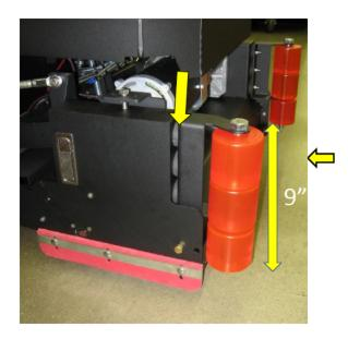
The MiniMag scrubber has shock mounted tower rollers on the cylindrical deck to absorb front collisions. A unique feature that protects both the machine and the customer's walls.
