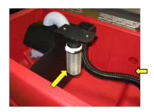
The MiniMag scrubber uses a stainless steel vacuum / foam protection screen, which can be cleaned and used for years, not the less expensive plastic options. Our intent is that this will save the customer money.
