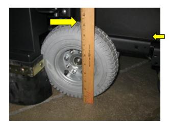
The MiniMag scrubber's have large diameter tires. The larger diameter improves the ride over expansion joints and irregular concrete surfaces. The tires have an aggressive tread pattern for improved traction and control.
