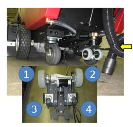
MiniMag scrubber has a 4-point stance for stability over rough surfaces. By using a 4-point stance instead of only 3, the MiniMag also offers improved safety on turns.
