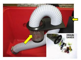
A feature to MiniMag scrubber is the "Drain Saver" stainless steel basket that collects litter from recovery water. This reduces the potential of discharge water clogging the customers' floor drains. A simple device that can avoid costly drain repairs for customers.
