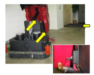
MiniMag Scrubber tank doesn't bolt to the frame, and so is less likely to be damaged or risk to stripped out inserts. The heavy duty and thick walled poly tank, pivots on smooth bosses.
