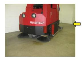
The heavy duty wide steel frame of the XR scrubber offers stability without the need for tip-over bars used on some other machines.
