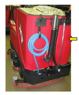
Spray Jet option equips the scrubber with a heavy duty hose 4' - 10' and spray nozzle. This allows the operator to use the scrubber's clean solution under pressure (3.0 gpm / 45 psi) to flush out the recovery tank when draining the tank when fresh water source is not within reach. Operator can also cleanout the scrub deck/hopper, pre-spray a large floor area for better detergent dwell time, cleaning under racks, around equipment, into restrooms and more.
