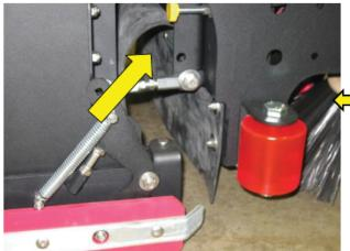
Unlike many other machines, the XR scrubber has a barrier to stop water or debris from being thrown onto the scrub deck.
