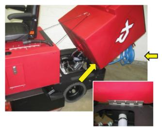
The XR scrubber uses larger (8" stainless) hinges and bolt directly into the heavy gage steel frame. This provides better durability than other machines that use smaller tank hinges bolted to plastic tanks.
