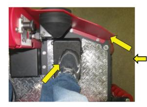
The XR scrubber has a simple and large pedal, which controls speed. This view also shows the protection offered to the Operator's foot on the XR scrubber. A complete apron across the front makes it harder for the operator to hang his foot off the side, reducing operator injuries.
