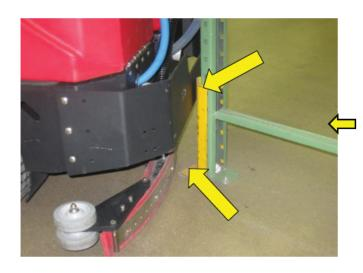
Our XR scrubber comes standard with a heavy-duty steel rear bumper, which helps protect the squeegees in "reverse" collisions. All scrubbers offer "breakaway" squeegees for "forward" collisions.
