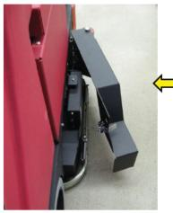
Side Doors are heavy gage, powder painted steel doors, which hinge open to access the scrub deck. These HD doors mount with a stainless hinge, to the rider scrubber's steel frame, and protect the scrub deck from collisions into poles, pallets and such. The doors include tall tower rollers, with non-marking polyurethane rollers, which spread impacts better and are less likely to damage or mark drywall.
