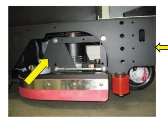
The XR scrubber uses durable, heavy-duty steel trailing arms and scrub deck, which are better able to withstand collisions and be repaired in the field than machines with plastic trailing arms and cast aluminum scrub decks.
