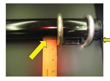
The XR scrubber 2" axle is larger than axles on many other machines. The larger axle is designed to support the XR scrubber in harsh applications and last the life of the machine.
