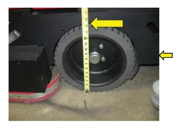
XR scrubber's have a 14" diameter tire. The larger diameter improves the ride over expansion joints and irregular concrete surfaces. Each tire is rated at 3,100 lbs, which is 3 times greater than the load with full tanks..
