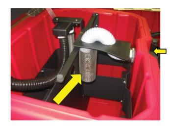
A feature to our XR scrubber is the "Drain Saver" stainless steel basket that collects litter from recovery water. This reduces the potential of discharge water clogging the customers' floor drains. A simple device that can avoid costly drain repairs for customers.
