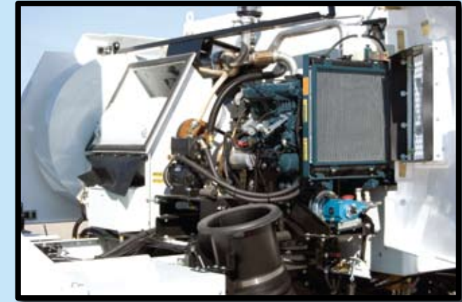
Locking side panels swing away for easy access to the auxiliary engine and blower housing.
