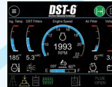
The high resolution color touchscreen display delivers on-board diagnostics for the TYMCO BlueLogic® Control System and the auxiliary engine's ECU (Engine Control Unit). Service reminders are displayed for the auxiliary engine and hydraulic system fluids and filters.
