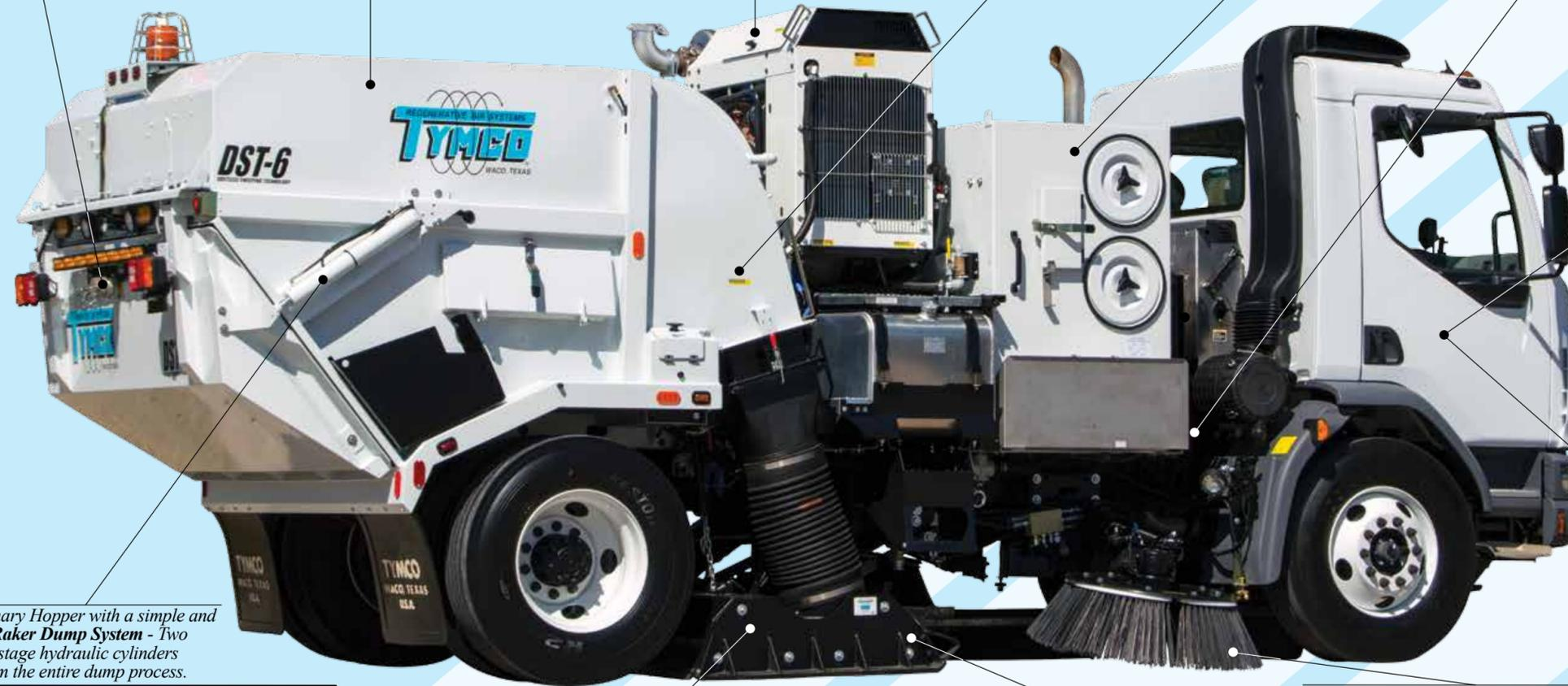
Stationary Hopper with a simple and safer Raker Dump System - Two single stage hydraulic cylinders perform the entire dump process.
